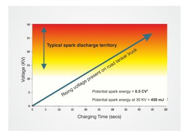
2. Voltage build-up on charged tank truck.
